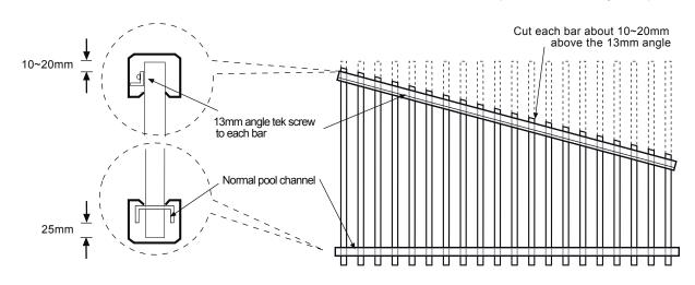
P10\_ ASSEMBLING PANELS WITH SLOPING TOP RAIL\_ 2.0
